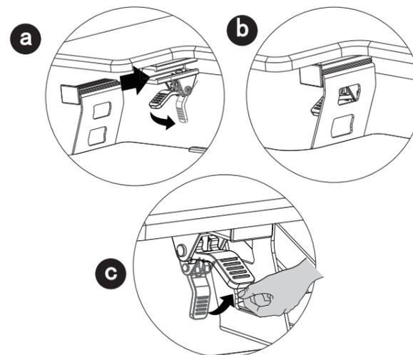
When removing the keyboard tray, please open the wrench and remove it. **!**
