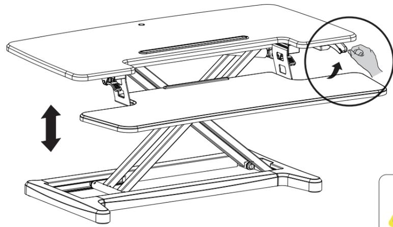
Based on the actual usage, press the handle on one side, and adjust the workstation to the proper height
